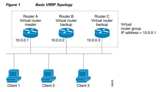
Because the virtual router uses the IP address of the physical Ethernet interface of Router A, Router A assumes the role of the *virtual router master* and is also known as the *IP address owner*. As the virtual router master, Router A controls the IP address of the virtual router and is responsible for forwarding packets sent to this IP address. Clients 1 through 3 are configured with the default gateway IP address of 10.0.0.1.
