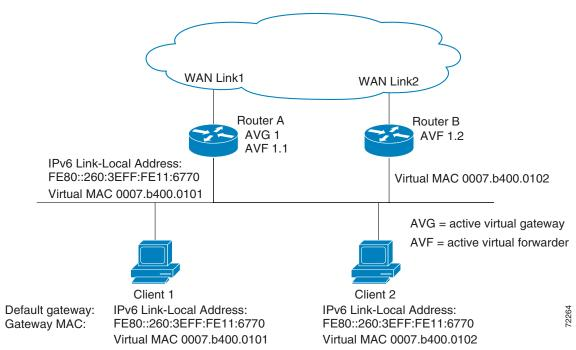
If Router A becomes unavailable, Client 1 will not lose access to the WAN because Router B will assume responsibility for forwarding packets sent to the virtual MAC address of Router A, and for responding to packets sent to its own virtual MAC address. Router B will also assume the role of the AVG for the entire GLBP group. Communication for the GLBP members continues despite the failure of a router in the GLBP group.
