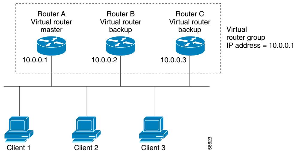
Because the virtual router uses the IP address of the physical Ethernet interface of Router A, Router A assumes the role of the *virtual router master* and is also known as the *IP address owner*. As the virtual router master, Router A controls the IP address of the virtual router and is responsible for forwarding packets sent to this IP address. Clients 1 through 3 are configured with the default gateway IP address of 10.0.0.1.
