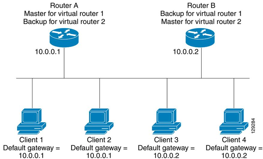
In this topology, two virtual routers are configured. (For more information, see the [“Multiple Virtual Router Support”](#) section later in this document.) For virtual router 1, Router A is the owner of IP address 10.0.0.1 and virtual router master, and Router B is the virtual router backup to Router A. Clients 1 and 2 are configured with the default gateway IP address of 10.0.0.1.
