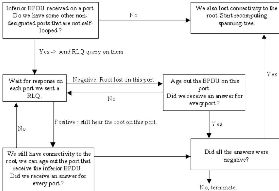
On receipt of an inferior BPDU from a designated bridge, send a RLQ PDU on all non-designated ports except the port where you received the inferior BPDU and self-looped ports. This is in order to check that you still hear from the root on ports where you are used to receiving BPDUs. The port where you received the inferior BPDU is excluded because you are already aware that it suffered from a failure, self-looped and
