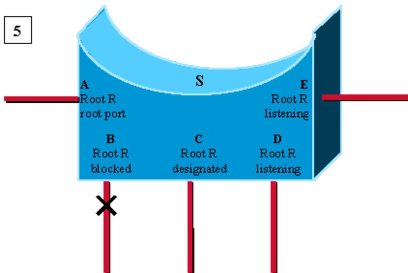
Port E transitions to listening, without waiting for max\_age. Usual spanning-tree rules then apply to determine whether E and D will eventually go to blocking or forwarding.
