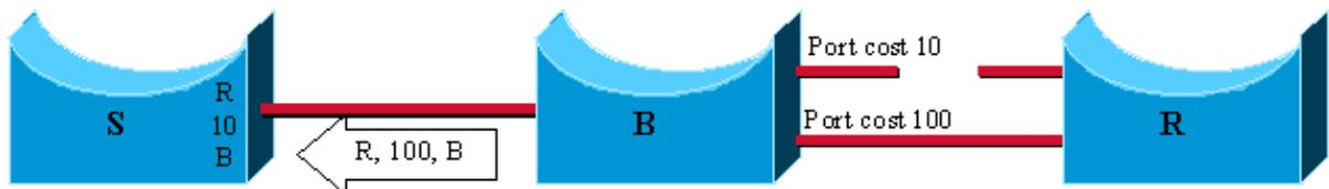
**2** In this case, B still has the root R, but the failure implied the cost to increase from 10 to 100. The BPDU sent is, again, inferior to the one stored by S (path cost 100 > value stored = 10)
