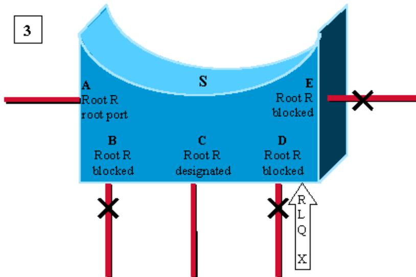
Port D is the first to receive an RLQ response from bridge X claiming to be the root. It is a negative response: D has lost connectivity to the root R. We age out immediately the BPDU on port D and go to listening. As we don't know if we still have connectivity to the root R, we don't age out port E yet.
