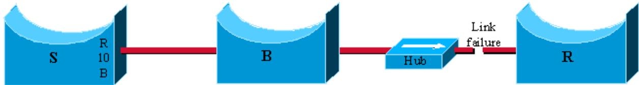
The link failure occurs between the root bridge R and the hub. B does not detect that the link goes down and waits max\_age before it claims to be the new root. Remember that the mechanism only works if a bridge detects a direct link failure.
