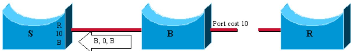
**1** In this case, B lost the root and sends a BPDU with root id B, path cost 0 and bridge id B. It is inferior to the one that S had stored, because R is a better root than B.
