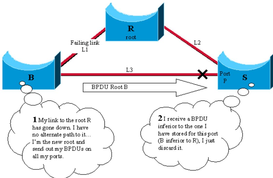
Consider this diagram, which involves three switches R, B, and S in a fully meshed topology. Assume that R is the root bridge and B is the backup root bridge. S blocks its port P and B is the designated bridge for link L3.
